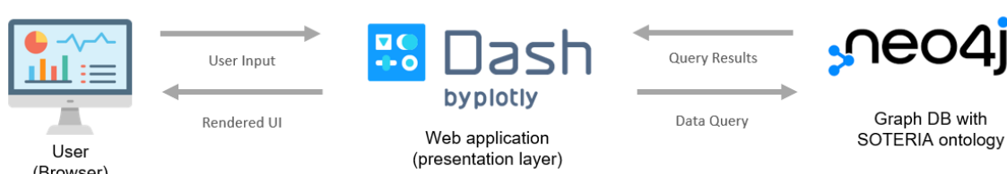
Figure 7: Overview of prototype architecture.
